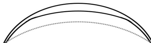
*Edge reduction for plus lenses with a soft overlap from optical zone to carrier. The optical zone will be adjusted according to power and frame shape.*
